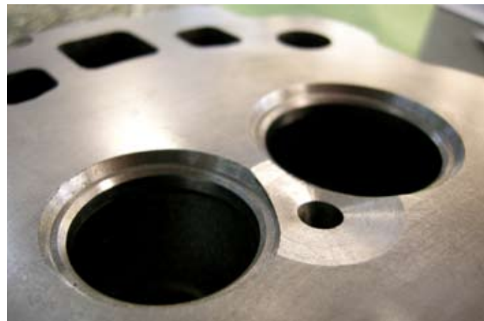
Stainless steel valves increase cylinder head durability.
